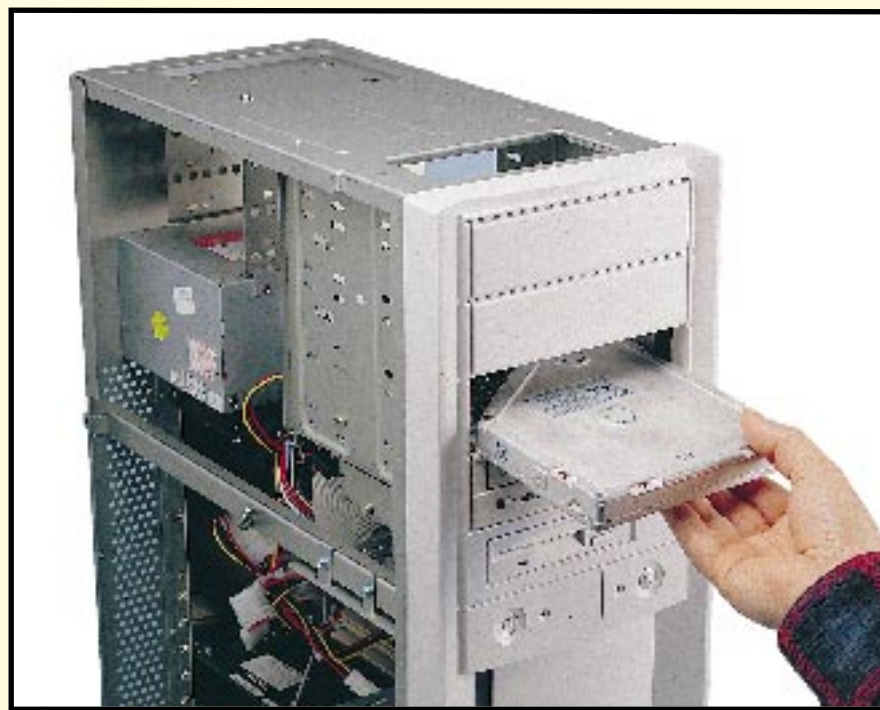
The Quantum Bigfoot is different to other EIDE drives as it will fill a 5.25in drive bay
